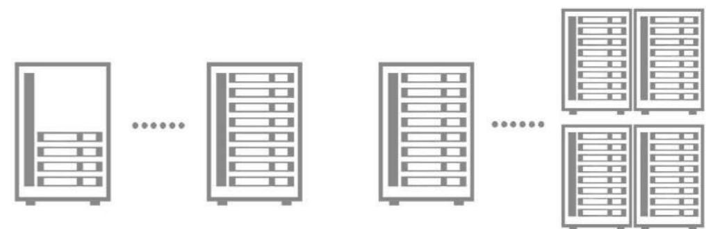
**Note:** Flexible Capacity Configuration: Pack Qty 4 to 8 into Cabinet adaptive to 600 - 1500V system.
